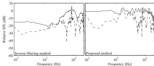
**Fig. 14** Frequency response functions from the desired signal  $r_1$  to the right ear  $y_{p1}$  (solid line) and left ear  $y_{p2}$  (dashed line) with movement of 6 cm of the head.
