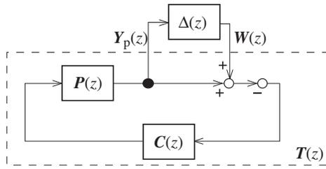
**Fig. 3** Closed-loop system with multiplicative plant uncertainty.
