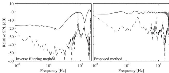
**Fig. 12** Frequency response functions from the desired signal  $r_1$  to the right ear  $y_{p1}$  (solid line) and left ear  $y_{p2}$  (dashed line) without movement of the head.
