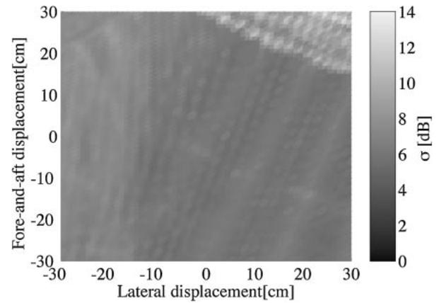
Fig. 17 Relationship of performance index  $\sigma$  to movement of the head for the inverse filtering method.
