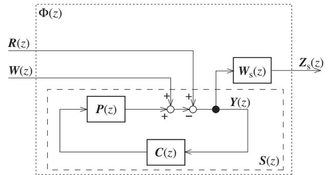
**Fig. 6** System configuration for disturbance attenuation and tracking problem.
