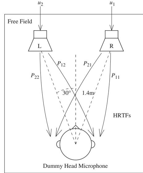
Fig. 9 Geometrical arrangement of loudspeakers and dummy head for cross-talk cancellation.
