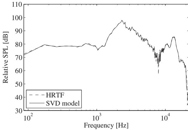
**Fig. 10** Frequency response functions of HRTF and its SVD model.
