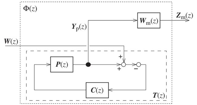
**Fig. 4** System configuration for robust stability problem.
