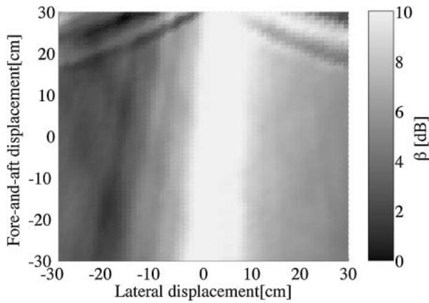
Fig. 16 Relationship of performance index  $\beta$  to movement of the head for the proposed method.
