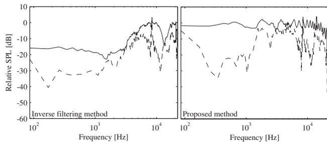
**Fig. 13** Frequency response functions from the desired signal  $r_1$  to the right ear  $y_{p1}$  (solid line) and left ear  $y_{p2}$  (dashed line) with movement of 3 cm of the head.
