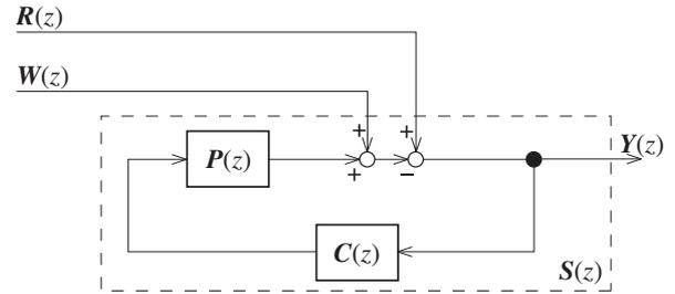
**Fig. 5** Closed-loop system excited by disturbance and desired signal.
