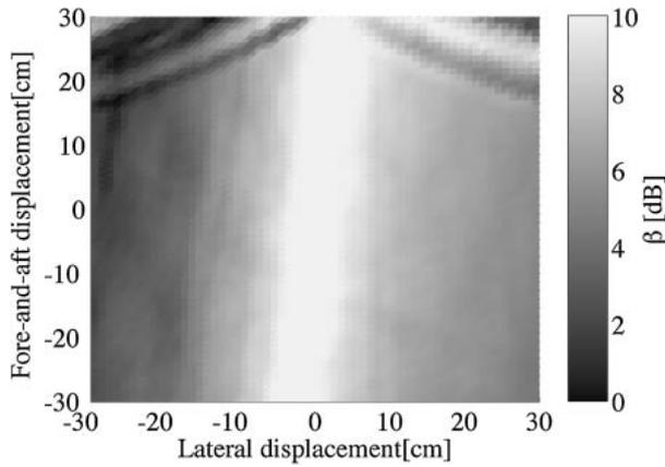
Fig. 15 Relationship of performance index  $\beta$  to movement of the head for the inverse filtering method.
