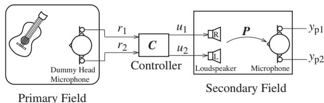
**Fig. 1** Arrangement of transaural system.
