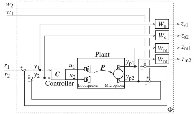
Fig. 8 Arrangement of proposed transaural sound reproduction system.
