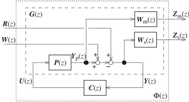
Fig. 7 System configuration for mixed sensitivity problem.
