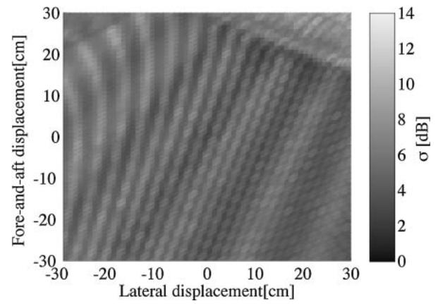
Fig. 18 Relationship of performance index  $\sigma$  to movement of the head for the proposed method.
